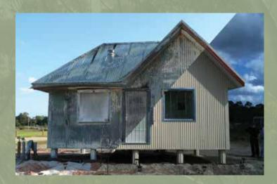
Warrior FZ Bushfire shutters are the only shutter available that have passed the AS1530.8.2 test without a window behind it. Typically, a shutter with a toughened safety glass window or door behind the shutter will contribute to the fire resistance of the shutter in the test.
